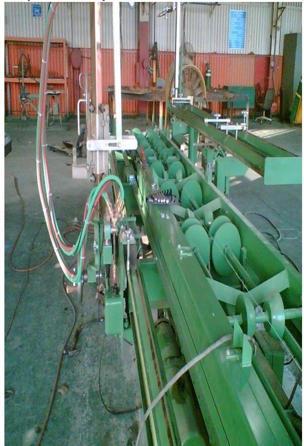
Installation of Pantograph Machine
